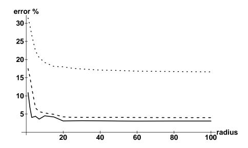
Figure 11: Perimeter estimation of circles in 3-D using link counting estimators. Average absolute errors (of 100 experiments) as a function of radius are compared. The dotted curve refers to the biased 26-directional link counting estimator. The dashed and solid curves respectively refer to the unbiased 26-directional and 6-directional link counting estimators, both developed in this paper.
