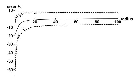
Figure 9: Perimeter estimation of circles in 3-D using the unbiased 26-directional link counting estimator developed in this paper. The solid curve shows the average error (of 100 experiments) as a function of radius. The dashed curves show the minimum and maximum errors encountered.
