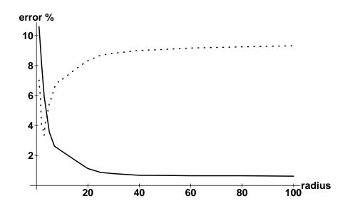
Figure 14: Perimeter estimation of circles in 3-D using link classification estimators. Average absolute errors (of 100 experiments) as a function of radius are compared. The dotted curve refers to the biased 26-directional link classification estimator. The solid curve refers to the unbiased, minimum RMS error, 26-directional link classification estimator developed in this paper.
