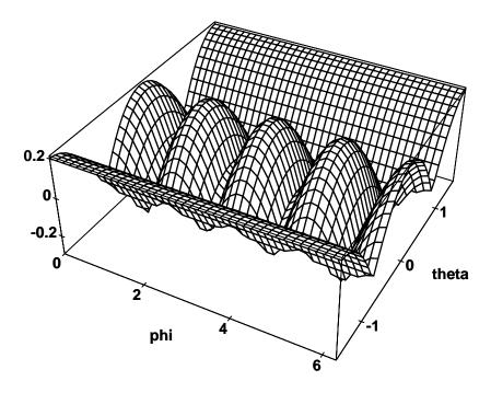
Figure 4: The dependence of the estimation error (in the case of straight lines) on  $\varphi$  and  $\theta$  for the unbiased 26-directional link counting estimator.
