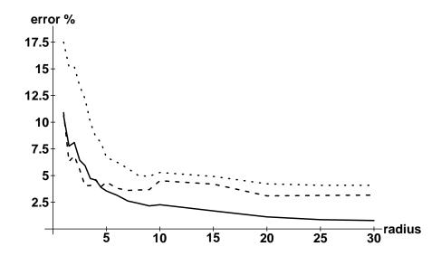
Figure 15: Perimeter estimation of circles in 3-D using the unbiased estimators developed in this paper. Average absolute errors (of 100 experiments) as a function of radius are compared. The dotted and dashed curves respectively refer to the unbiased 26-directional and 6-directional link counting estimators. The solid curve refers to the unbiased, minimum RMS error, 26-directional link classification estimator.
