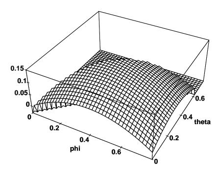
Figure 6: The dependence of the estimation error (in the case of straight lines) on  $\varphi$  and  $\theta$  for the biased link classification estimator. The typical domain  $0 \le \varphi \le \pi/4$ ,  $0 \le \theta \le \arctan \sin \varphi$  is shown. The error is non-negative, i.e., the length is never underestimated.
