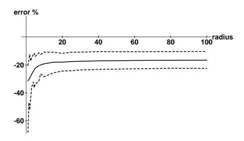
Figure 8: Perimeter estimation of circles in 3-D using the biased 26-directional link counting estimator. The solid curve shows the average error (of 100 experiments) as a function of radius. The dashed curves show the minimum and maximum errors encountered.
