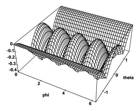
Figure 3: The dependence of the estimation error (in the case of straight lines) on  $\varphi$  and  $\theta$  for the biased 26-directional link counting estimator. The error is non-positive, i.e., the length is never overestimated.
