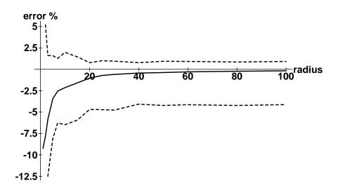
Figure 13: Perimeter estimation of circles in 3-D using the unbiased, minimum RMS error, 26-directional link classification estimator developed in this paper. The solid curve shows the average error (of 100 experiments) as a function of radius. The dashed curves show the minimum and maximum errors encountered.
