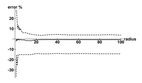
Figure 10: Perimeter estimation of circles in 3-D using the unbiased 6-directional link counting estimator developed in this paper. The solid curve shows the average error (of 100 experiments) as a function of radius. The dashed curves show the minimum and maximum errors encountered.
