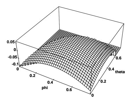
Figure 7: The dependence of the estimation error (in the case of straight lines) on  $\varphi$  and  $\theta$  for the unbiased link classification estimator. The typical domain  $0 \le \varphi \le \pi/4$ ,  $0 \le \theta \le \arctan \sin \varphi$  is shown.
