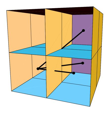
Figure 1: Link types in a 26-directional 3-D chain code: a direct link (parallel to one of the main axes), a minor diagonal link and a major diagonal link.
